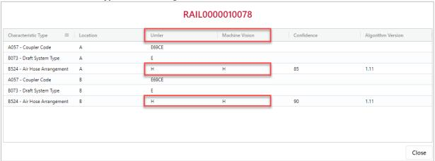
7. A flag appears in the **Flag** column when <u>Machine Vision data does not match Umler data</u>. In the example below, Air Hose Arrangement A and B data for Machine Vision does not match with Umler.
